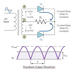
During the positive half cycle of the supply, diodeD1 conducts , while diodeD2 is reverse biased and the current flows through the load as shown .
