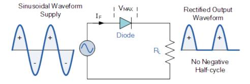
Here – ve half cycles are suppressed i.e. during –ve half cycle no current passes through the diode hence no voltage appears across the load.
