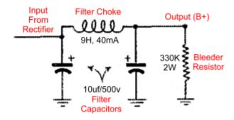
In this filter one inductor & two capacitors are used.
