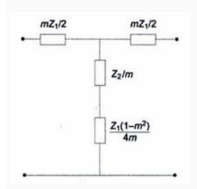
The characteristic impedances of the prototype and its modified sections have to be equal for matching.
