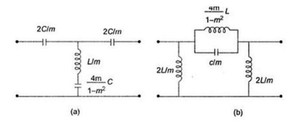
the m-derived \[\pi\]-section, the resonant circuit is constituted by the series arm inductance and capacitance.
