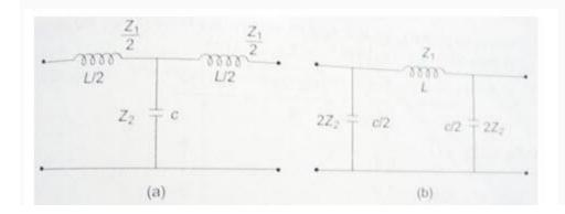
where  $Z_1 = j\omega_L$  and  $Z_2 = 1/j\omega_C$ . Hence  $Z_1Z_2 = \{\{L \mid C\}\}\}$  which is independent of frequency
