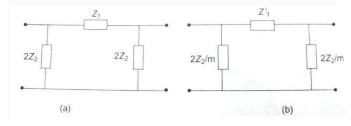
the characteristic impedance of the modified (m-derived) \[\pi\]-network
