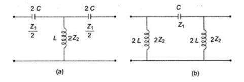
Again, it can be observed that the product of  $Z_1$  and  $Z_2$  is independent of frequency, and the filter design obtained will be of the constant k type.
